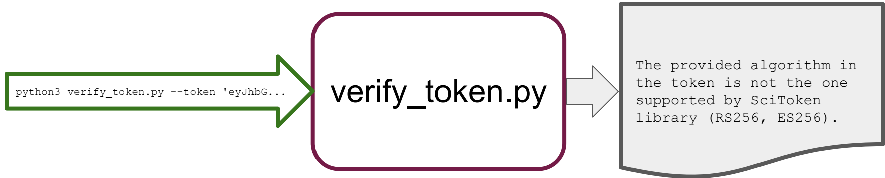
Figure: Workflow of python based test suite to verify SciTokens
